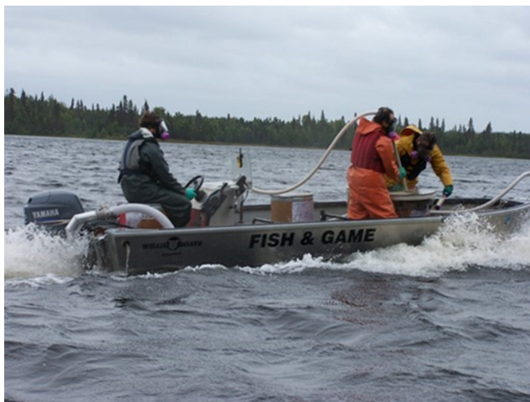
SOP7.5. Outboard boat applicators applying powdered piscicide by siphoning the powder from a drum with a probe (aluminum tube) that is connected by hose to an eductor that is powered by pump discharge. The eductor premixes the powder with lake water and discharges the slurry through a hose attached near the boat's bow. Three applicators are shown working, one as the boat operator, a second to control the siphon probe, and a third to break-up clumped powder by agitating the piscicide drum with a bat so it can be siphoned more easily
