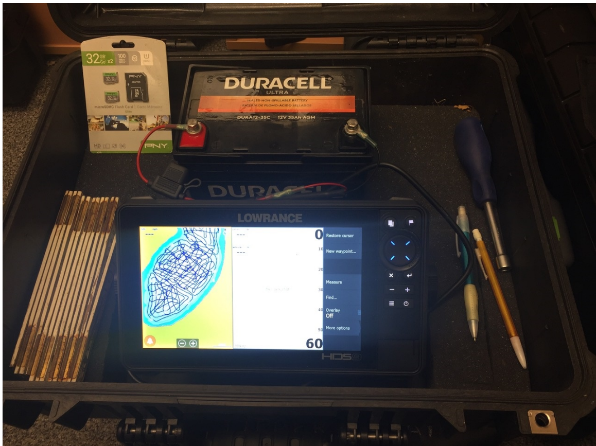
SOP 6.3. Example of the pelican case set up for the mapping unit
