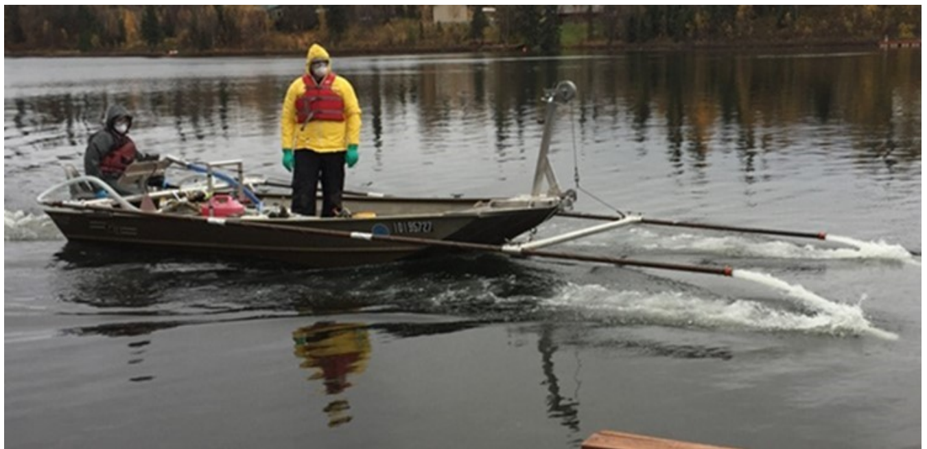
SOP7.3. Rotenone application boat that is custom equipped for deep water applications. Rotenone premixture is discharged from pipes that can be lowered 18-feet below the water surface using a hand-operated winch and bridle assembly. The use of weighted hoses can also be used to apply rotenone to deep water strata to promote better piscicide distribution. Underwater drag on submerged pipes or hoses require a much slower boat speed
