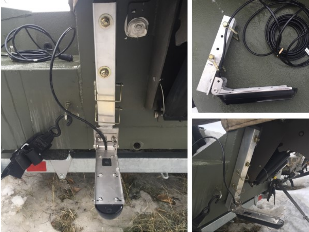
SOP 6.1. Transducer mounted to a boat
