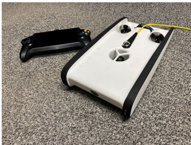
SOP8.1. Submersible drone ROV that can be used for under-ice net checks and deployment
