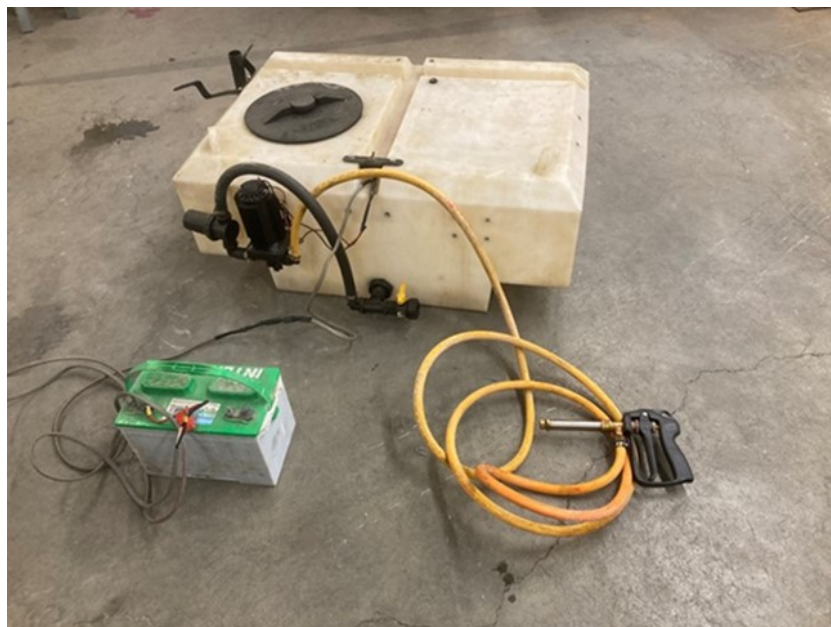
SOP7.7. Battery-powered (12-volt) on-demand hand-held sprayer gun with a 45-gallon mixing tank. When applying piscicide in large areas of dense aquatic vegetation and/or shallow mucky areas, a mixing tank filled with a piscicide premixture can eliminate pump clogging issues common to gas-pump systems. A mixing tank is ideally used with a non-outboard watercraft (i.e., canoe, airboat) that reduces disturbance to lake sediments. Suspension of organic sediment can reduce rotenone's efficacy
