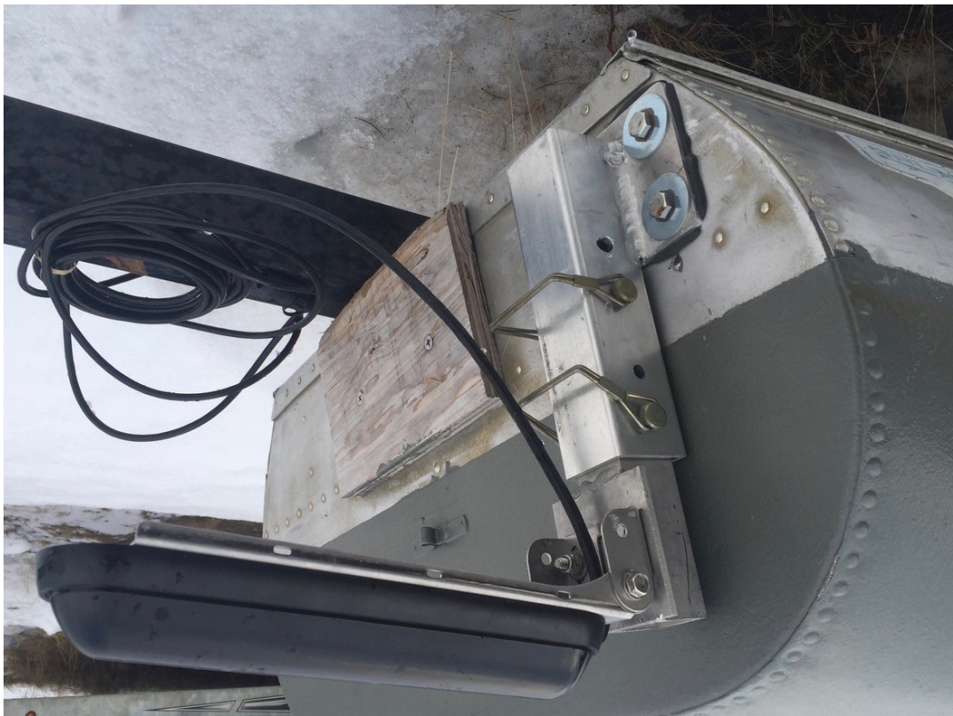
SOP 6.2. Transducer mounted to a canoe
