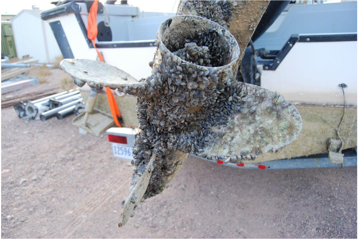
Zebra mussel fouled propeller from Lake Mead, Arizona. Photo credit: NPS.
